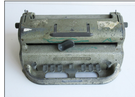
Braille Typewriter, Perkins Brailler Manual Mechanical Braille Printer from 1951
